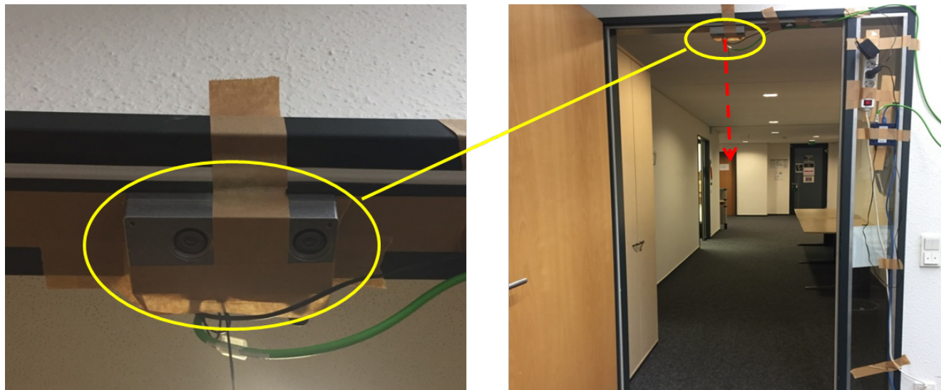
Figure 4. Lab experiments with stereoscopic camera. Left: The camera on the office room door. Right: The viewing angle of the camera.
